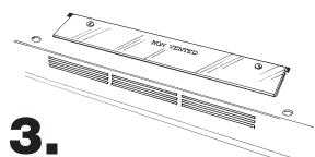
Remove screws from vent baffle on top of range hood. Remove vent baffle.
